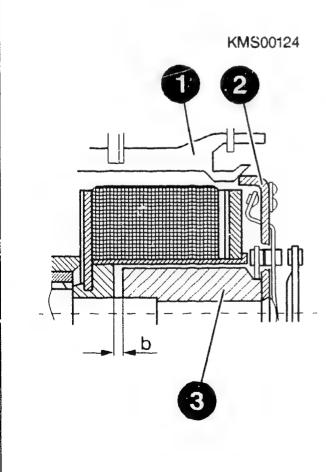
CHECKING AND REPAIRING COMPONENTS Checking return force of helical spring on engaging shaft This is performed with startingmotor assembled. It must be possible to push pinion back into rest position with spring action via rubber buffer in thrust piece of starting-motor solenoid. Engaging shaft must be seated on ball (1) in starting-motor solenoid in rest position. Initial force: 50...60 N 71...81 N Final force:
